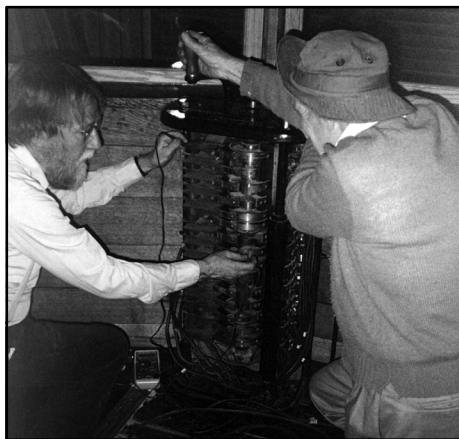
Carlos Seegmiller (left) and Des Sainsbury test the controller circuits on the number two end of the No. 25 in early April. – Darrell Arndt Photo
