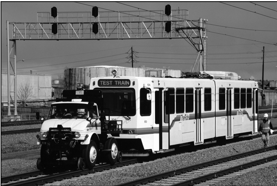
RTD car 104 was used as a test car to check clearances on the new Southwest Corridor. A hy-rail truck pulled the car on 4/2/00. – Photo © Chip Sherman
